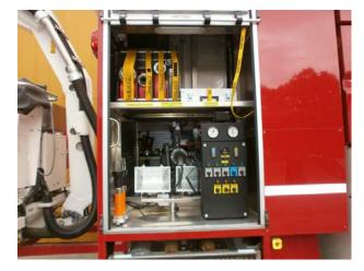
Side mounted pump control panel
