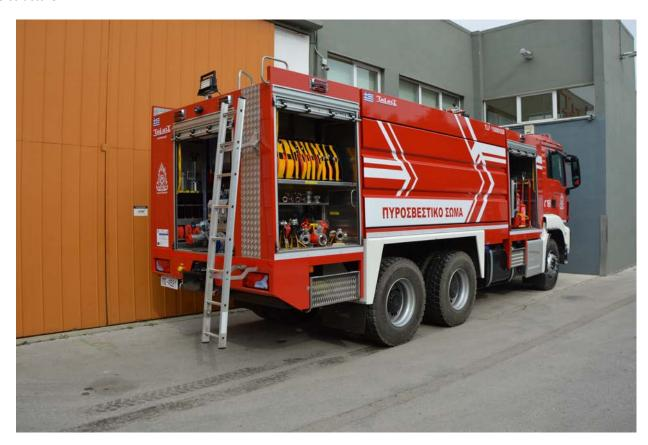
**Design:** Modular, with front equipment locker, full width water tank and rear pump locker.
